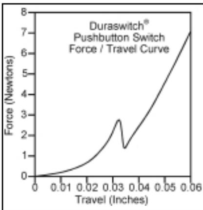
Figure 3: Duraswitch Pushbutton Switch Force/Travel Curve
