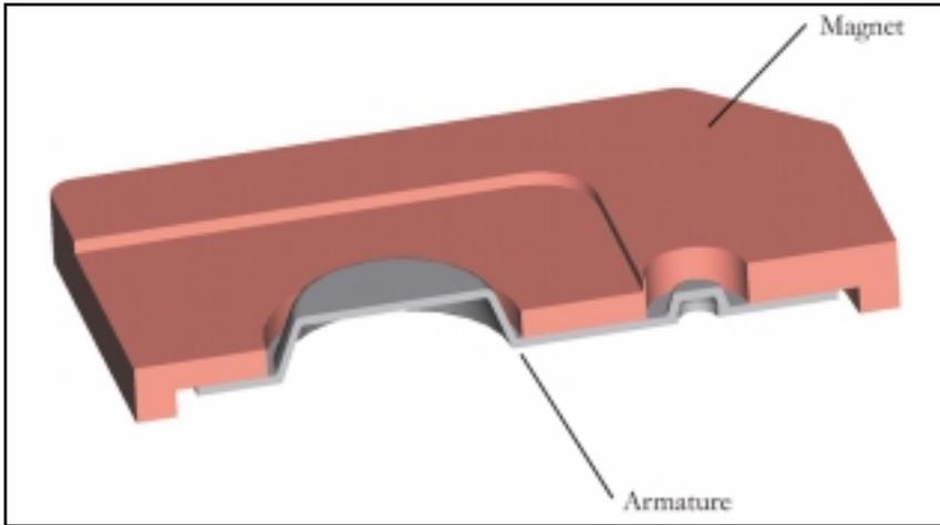
Figure 2: Duraswitch PushGate Island Switch
